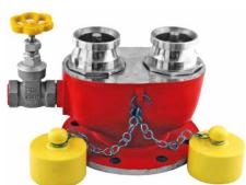
Fire Brigade Inlet (also called Pumping In Breech) allows Fire Tenders (Pumpers) to pump in water into the Dry Riser/ Wet Riser/ Sprinkler system piping using external water sources such as hydrants. Fire Brigade Inlet is fitted with required number of standard Male Instantaneous inlets to feed the Riser pipe depending upon size.
